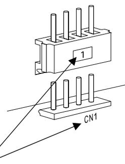
**NOTE: Match the number on the printed circuit board with that on the connector.**
