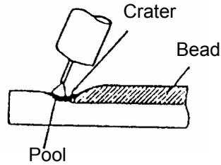
Crater is a depression left at the termination of the weld. As it may cause cracks and poor welding, a crater treatment called crater-filler is used to fill in the depression.
