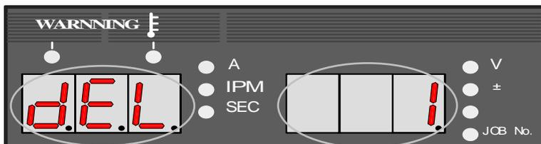
"dEL" display means the machine in the delete mode.
