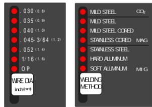
Set a welding method, then wire diameter by using the WELDING METHOD key, and the WIRE DIA. (In.) key respectively.
