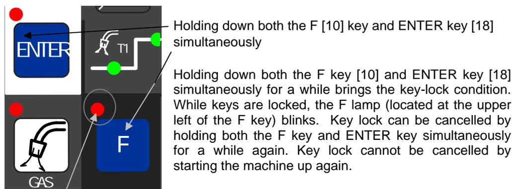
While keys are locked, the F lamp blinks
