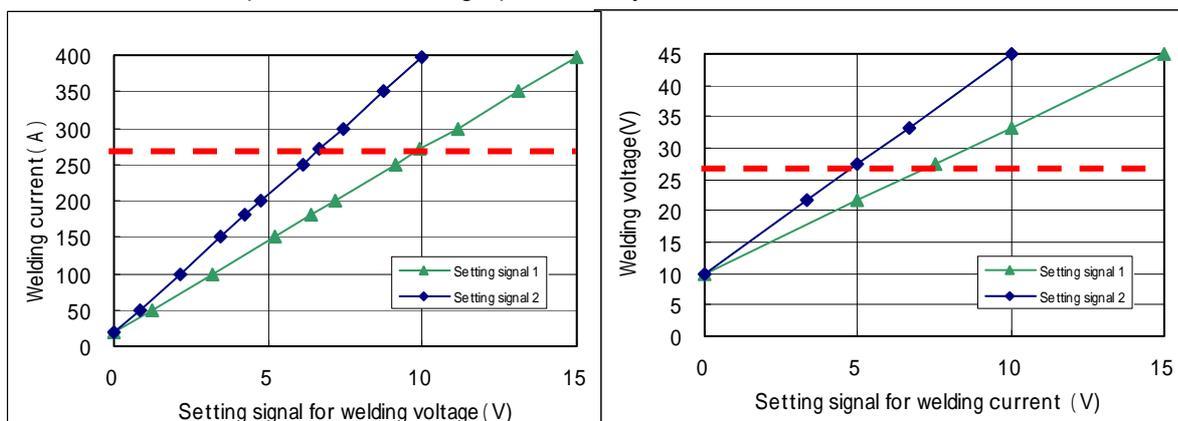
\* Setting Signal 1: When command voltage is externally supplied in the range from 0V to 15V under the standard settings.
