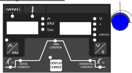
Use the DISPLAY CHANGE key to select the parameter you want to set, then adjust it while turning the parameter adjusting knob.
