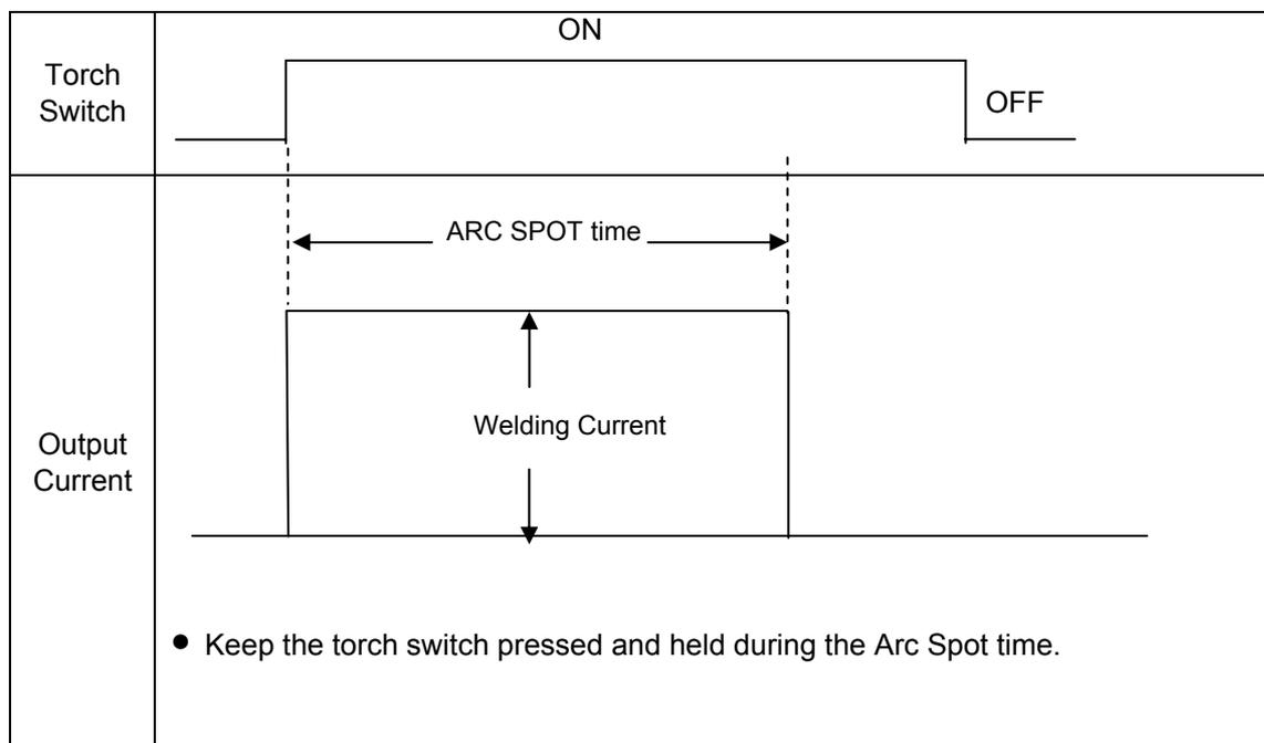
**NOTE: When the welding machine is in the ARC SPOT mode, the penetration control does not function. When setting the CRATER-FILL function to "SPOT" while the CONSTANT PENETRATION function is "ON", the setting of the CONSTANT PENETRATION function is automatically changed to "OFF".**
