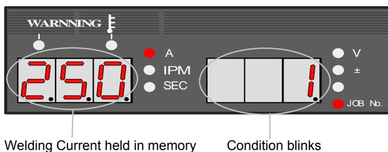
In the event that any memory data is preset to the condition number you selected, the CRATER lamp, the WELDING METHOD lamp, etc. also lights up. When no memory data is preset to the condition number, "- - -" in the left-side display appears and blinks. See the figure below.
